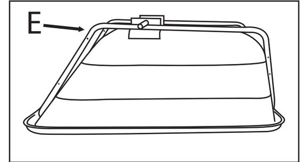
Take Cage Support Bottom (E) bars (2) and place them inside the Cage Support Front/Back Bars and connect with Screws (Part P) and nut. Do not tighten.
