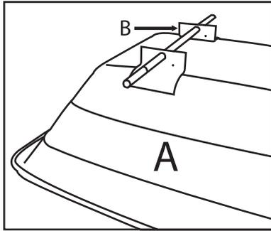
Turn Tub (A) upside down and place Axle (B) on top near the front end of the cart.
