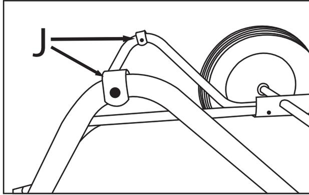
Add Skid Caps (J) to bottom of Legs using two Screws (Part Q).
