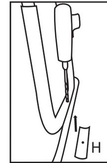
Make sure cage support system is centered and drill hole through plastic lip on each end of the cart using the holes in the support bars as a guide. Use Screws (Part R) to fasten frame to tub on both ends. Also, place Lip Protector (H) on top of lip on both ends before fastening.
