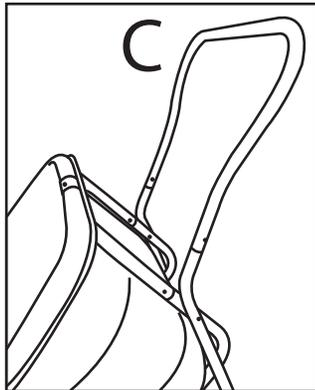
Add Handle Bar (C) and fasten with two Screws (Part P) and Wing Nut (Part L).
