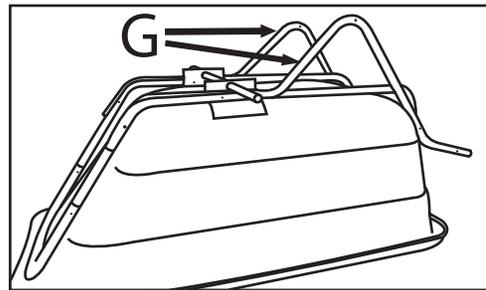
Place both Leg Support Bars (G) on outside of Cage Support bars. Secure Legs and Cage Supports to Axle Plate using 4 Screws (Part T). Also, connect Cage Support to Leg Supports using 4 Screws (Part S), Two in front, two in back. Snug ALL bolts at this time.
