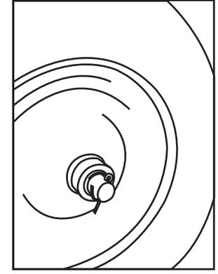
Add Cotter Pin (N) to each axle to secure wheels.
