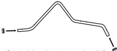
Place End Caps (Part K) into each end of the two Leg Support Bars.
